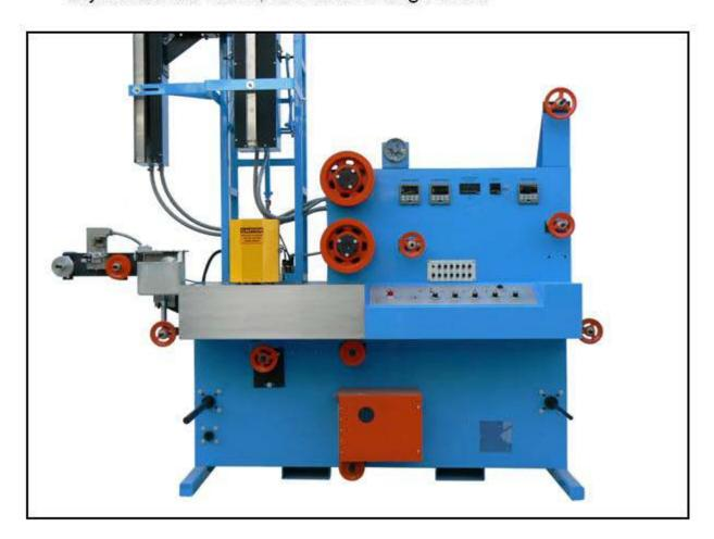
**Digital Display:** The digital readout indicates RPM of the striping head, FPM of wire and the ratio of the two, in stripes per foot (metric available).
